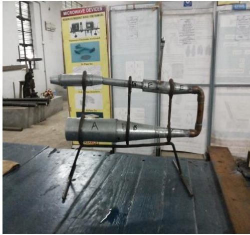
A prototype of a valve less pulse jet engine at an initial level.
