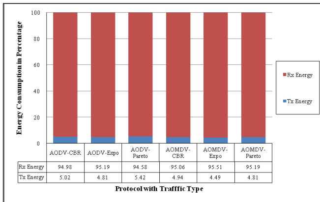
Figure 6: Energy consumption percentage of total transmission and receiving energy due to control packets with 50 nodes
