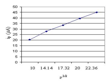
As significant peaks were missing in the cyclic voltammograms recorded in acidic condition, scan rate variation studies were done in neutral and alkaline media. In both cases a linear relationship is observed between log  $(i_{pa})$  and log  $\square$  (where  $i_{pa}$  is anodic peak current and  $\square$  is scan rate). Furthermore the plot between the peak
