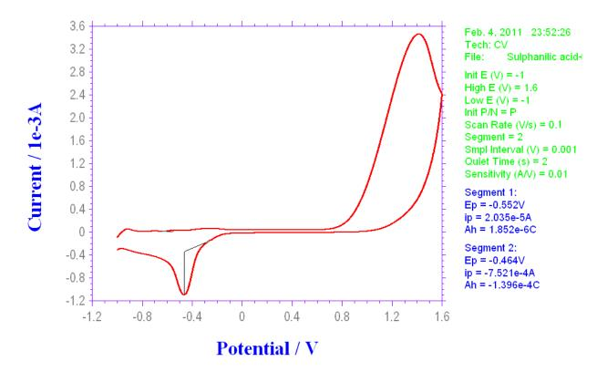
In neutral and alkaline condition the peak potentials were almost similar. The oxidation and reduction peaks obtained in the acidic condition were not as significant as they are found in the neutral and alkaline conditions. This is due to the difficulty in the formation of ethoxide ion and also due to the protonation of the medium to a greater
