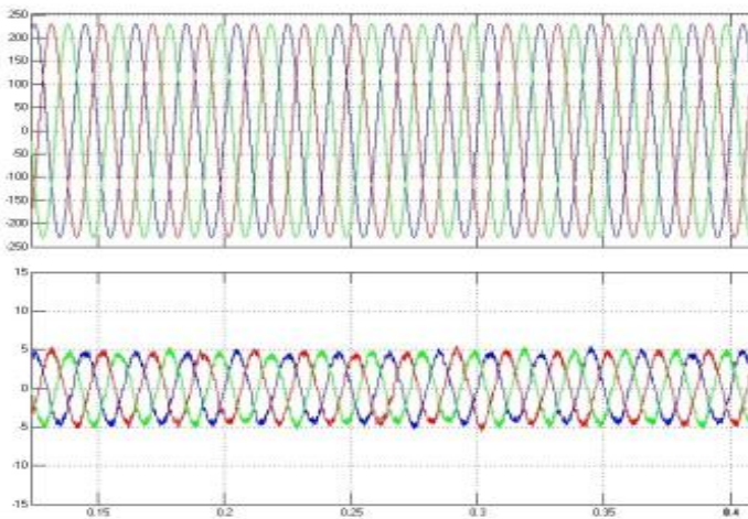
Fig.7 Input voltage and current waveform
