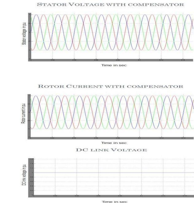
**Fig. 9.** Simulation results for a three-phase short circuit on the terminal of a 1.5-MW DFIG wind turbine when a full compensation is applied.
