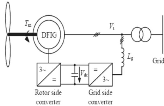
**Fig.3.** Configuration of a DFIG wind turbine system
