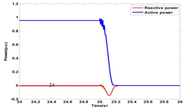
**Fig. 9.** Active and reactive power delivered with exponentially decaying voltage compensation ( $V_c = V_c e^{-t/ \tau 1}$ ).
