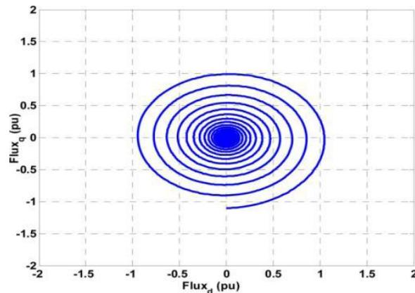
**Fig. 7.** Stator flux trajectory transients with compensation.
