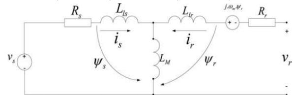
**Fig.4.** DFIG- equivalent circuit for short circuit analysis.
