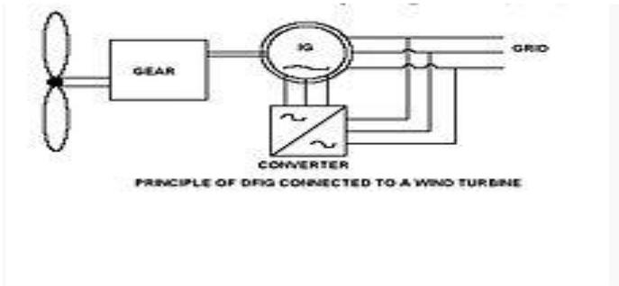
**Fig 2.1** Principle of a Double Fed Induction Generator connected to a wind turbine
