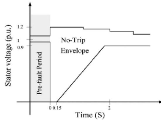
**Fig.1:** WECC voltage ride-through requirements for all generators. 494
