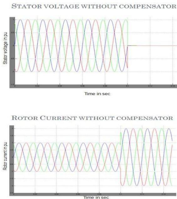
**Fig. 10.** Simulation results for a three-phase short circuit on the terminal of a 1.5-MW DFIG wind turbine.
