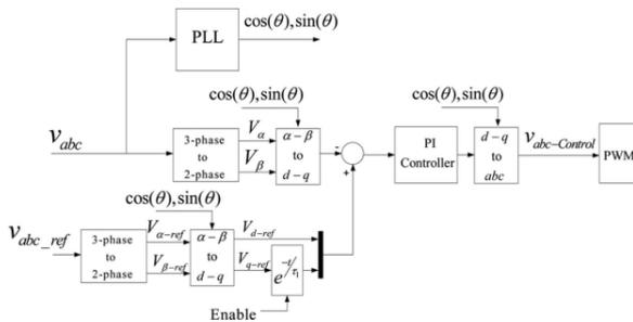
**Fig. 8.** Block diagram of the converter control technique.
