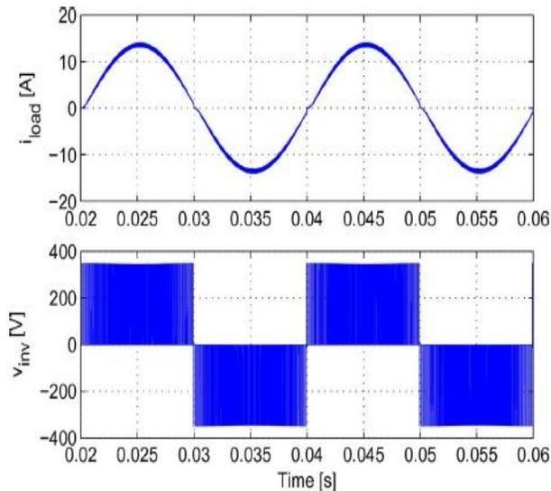
**Fig.10.** HERIC topology: Load current and inverter output voltage.
