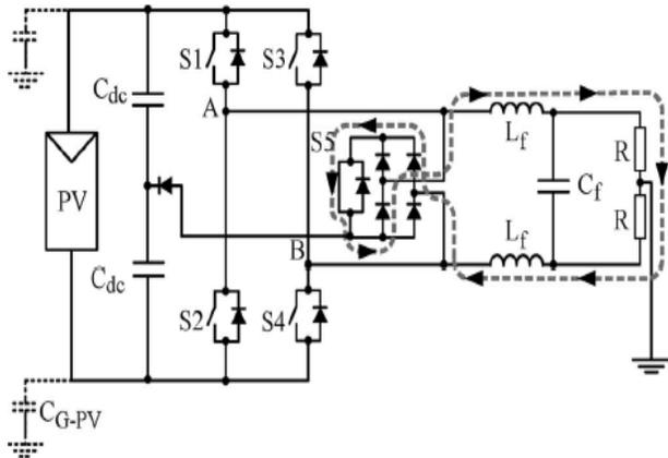
**Fig. 13.** HB-ZVR topology: Zero vector applied to load, using S5 during positive half-wave.
