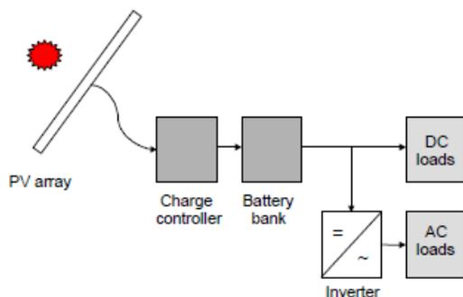
**Fig. 2** Schematic diagram of a stand-alone photovoltaic system
