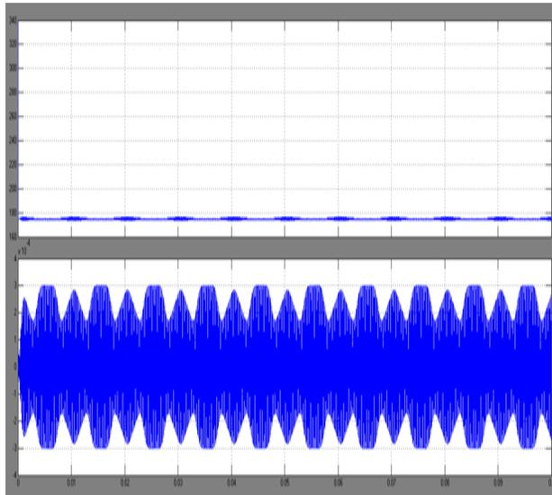
**Fig.20** common mode voltage ( $V_{pe+}$ ) and ground current ( $I_{gnd}$ )
