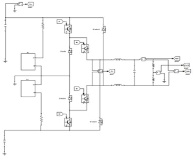
**Fig 17.** Midpoint Grounding HB with Unipolar Switching
