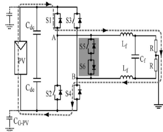
**Fig. 8.** HERIC topology: Active vector applied to load, using S1 and S4 during positive half-wave.
