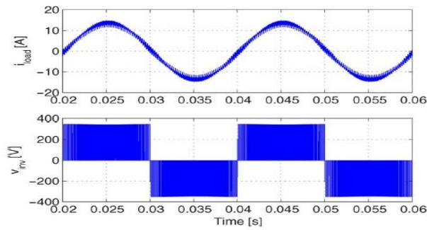
**Fig. 6.** HB-Unip topology: Load current and inverter output voltage
