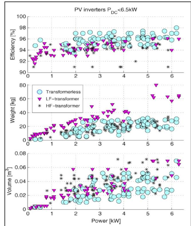
**Fig.1.** Advantages and drawback of different inverter topologies
