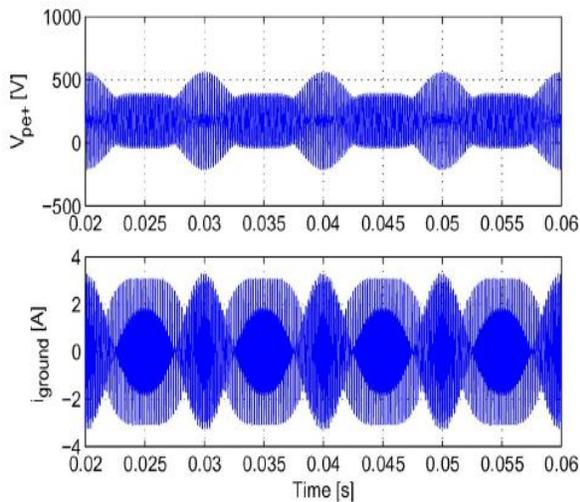
**Fig. 7.** HB-Unip topology: Voltage to ground and ground leakage current.
