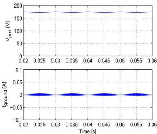
**Fig.11.** HERIC topology: Voltage to ground and ground leakage current.
