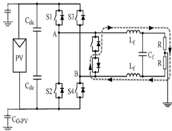
**Fig. 9.** HERIC topology: Zero vector applied to load, using S6 during positive half-wave.
