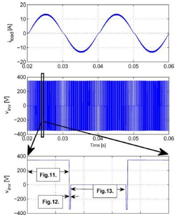
**Fig. 15.** HB-ZVR load current and inverter output voltage.
