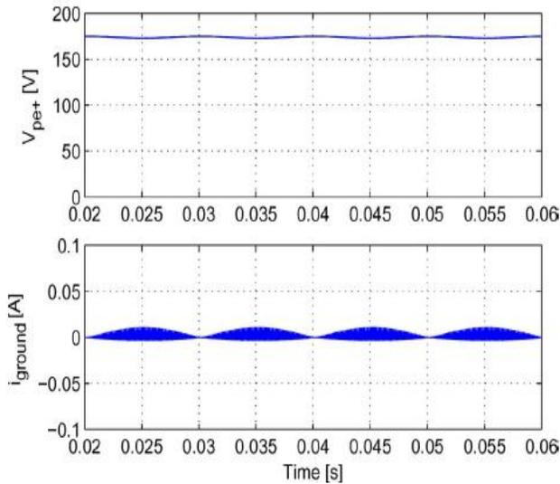
**Fig.16.** HB-ZVR topology: Voltage to ground and ground leakage current.
