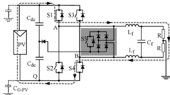
**Fig. 12.** HB-ZVR topology: Active vector applied to load, using S1 and S4 during positive half-wave.
