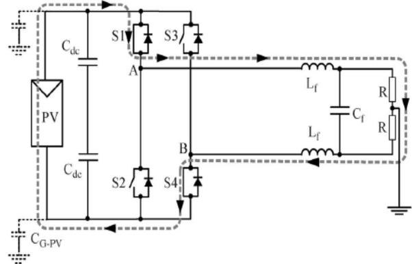
**Fig.4.** HB-Unip topology: Active vector applied to load, using S1 and S4 for positive voltage.
