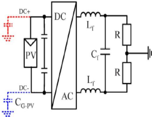
**Fig. 3.** Test setup used for common-mode voltage measurement.
