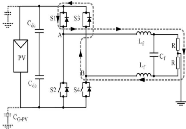
**Fig.5.** HB-Unip topology: Zero vector applied to load, using S1 and S3 for positive voltage.
