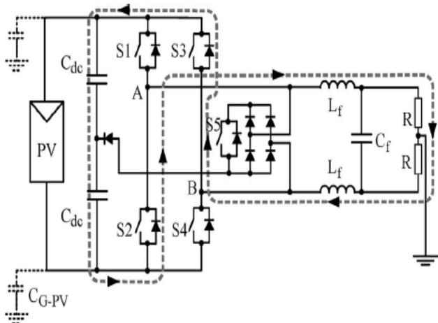
**Fig.14.** HB-ZVR topology: Dead time between turnoff of S1 and S4 and turn on of S5 during positive half-wave.
