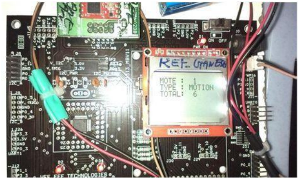
Figure 10: Monitoring mote displaying intrusion, Sample 1.
