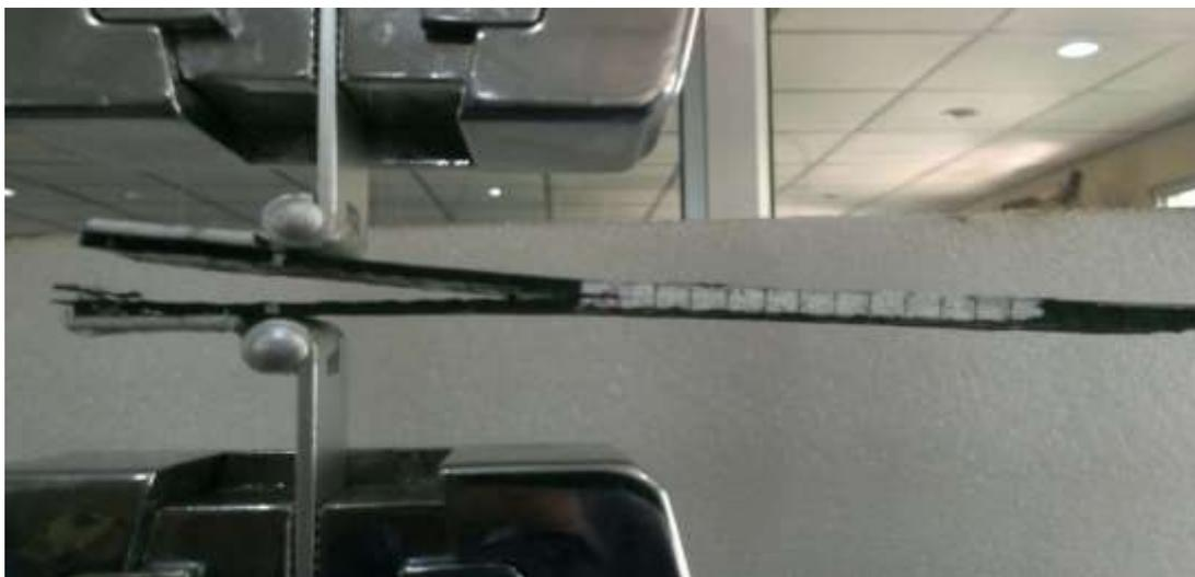
Fig.2. DCB test specimen in Universal Testing Machine
