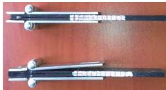
Fig.1. Double Cantilever Beam Specimen
