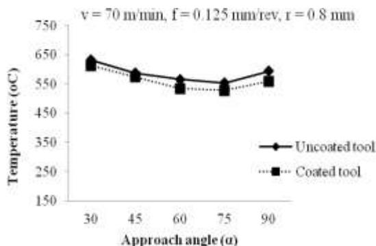
Fig-3(b): Variations of Cutting temperature with approach angle
