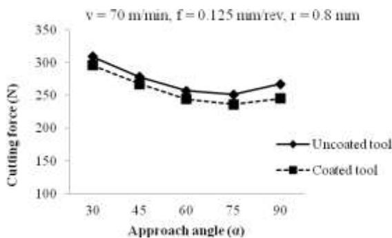
Fig -3(a): Variations of Cutting force with approach angle
