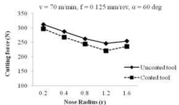
Fig -4(a): Variations of Cutting force with nose radius
