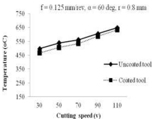
Fig -1(b): Variations of cutting temperature with cutting speed
