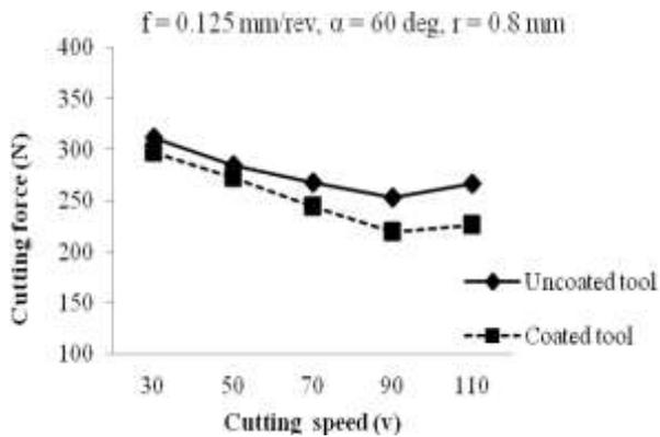
Fig -1(a): Variations of Cutting force with cutting speed
