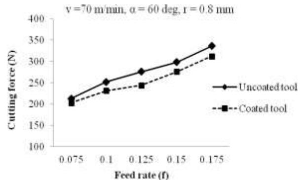
Fig -2(a): Variations of Cutting force with feed rate
