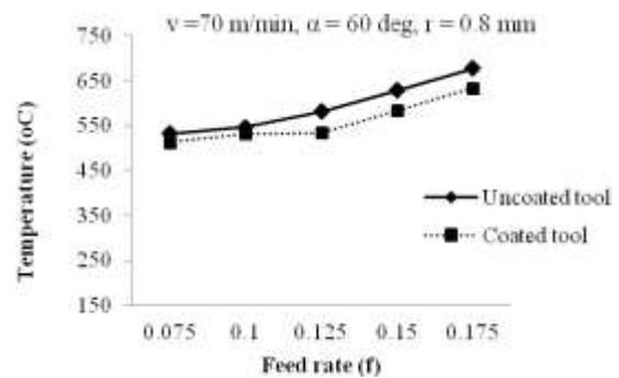
Fig -2(b): Variations of Cutting temperature with feed rate
