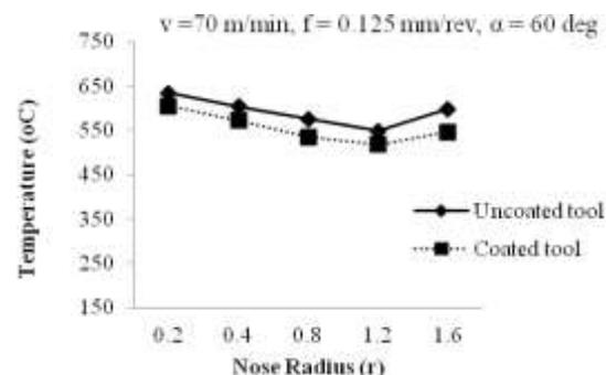
Fig-4(b): Variations of Cutting temperature with nose radius
