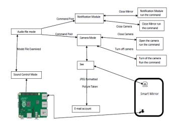
Figure 6. Block diagram of the mirror application
