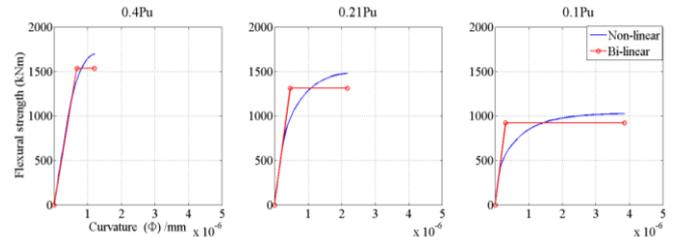
Fig. 8: Moment curvature relationship of wall A
