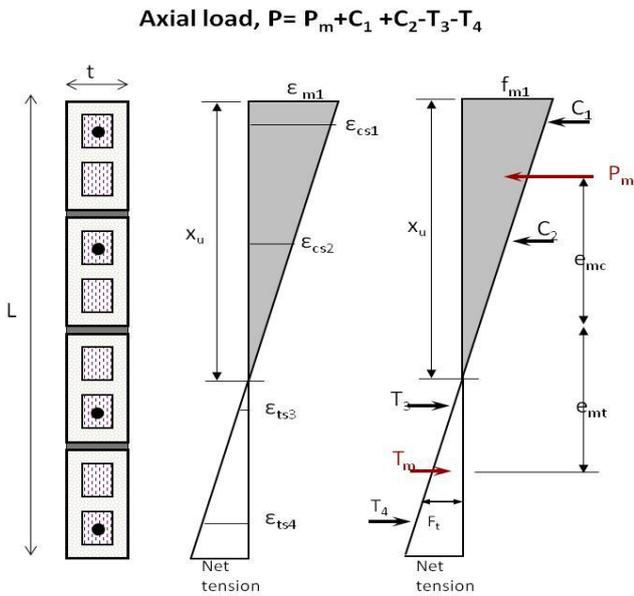
**Fig. 2.** Typical stress and strain distributions across rectangular RM walls A) Entire section under compression and B) Once tensile cracking commences
