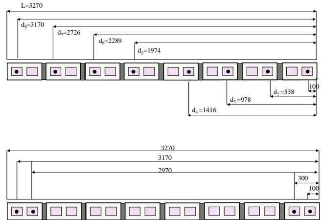
Fig. 6: Cross section of wall A uniformly distributed steel and wall B steel at corners
