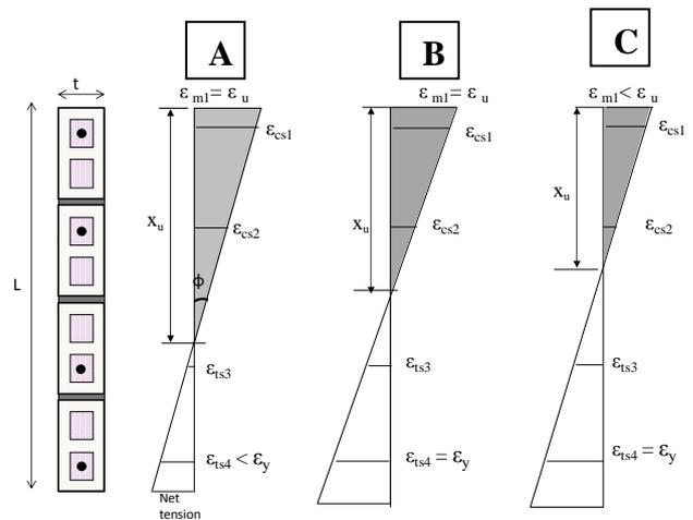
**Fig. 5:** Strain variations across RM sections under axial loads A) Above balance point B) At balance point C) Below axial load
