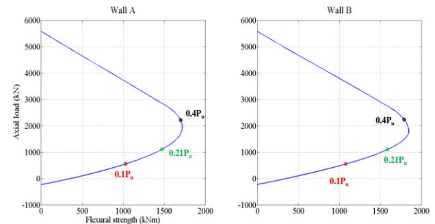
Fig. 7: Axial load –bending moment interaction diagram for the wall A and wall B
