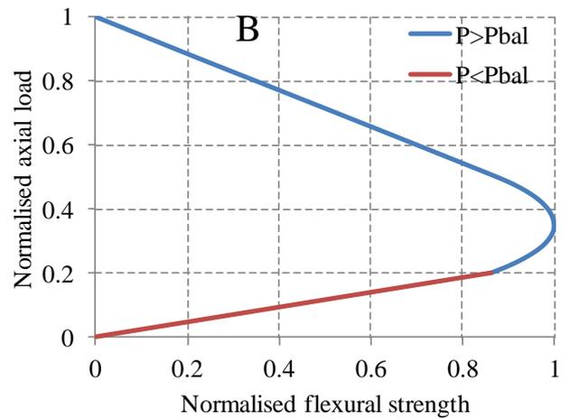
**Fig. 4:** Typical axial load-bending moment interaction of RM walls
