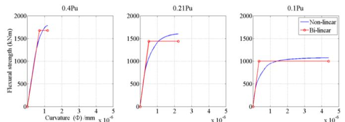
Fig. 9: Moment curvature relationship of wall B
