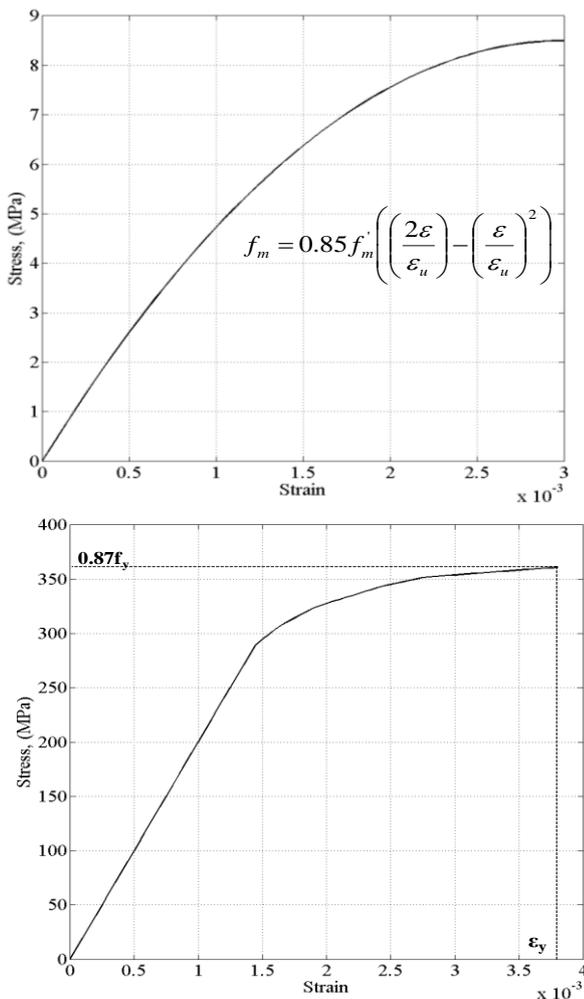
**Fig. 3:** Design stress-strain relation for A) masonry and B) reinforcing steel
