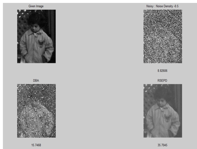
Figure 4. Results of SEPD in MATLAB, (a) Noise-free image; (b) Noisy image; (c) DBA; (d) Edge Preserved output
