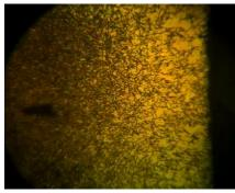
$4\,\%$  Nital etched sample shows carburizing case depth Upto  $0.6\,\mathrm{mm}$  at  $500\mathrm{X}$  magnification range.
