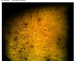
4 % Nital etched sample shows carburizing case depth Upto 0.8 mm at 500X magnification range. **SAE8620 GEAR**
