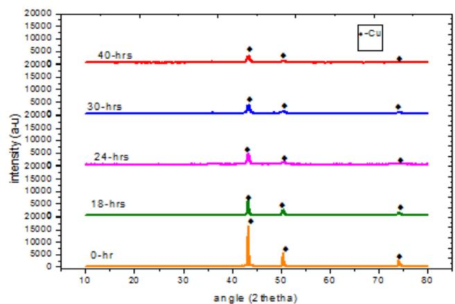
**Figure 1** XRD pattern of Cu powder as a function of milling time
