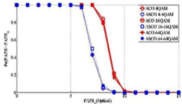
**Fig 2. PAPR (OPTICAL POWER) Comparisons Of 2D ASCO-OFDM And 2D ACO-OFDM**
