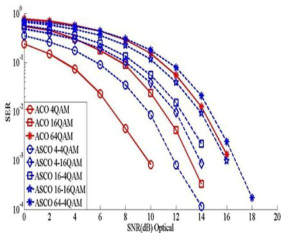
**Fig 3.** Ser Comparisons Of 2D ASCO-OFDM And 2D ACO-OFDM With Different Constellation Combination
