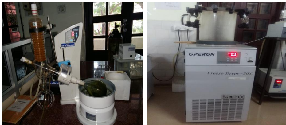
Fig 1: Showing rotary flash evaporator and freeze dryer
