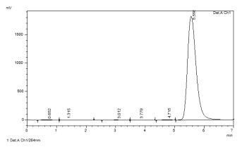
Fig 2 chromatogram showing the retention time for Pantoprazole standard
