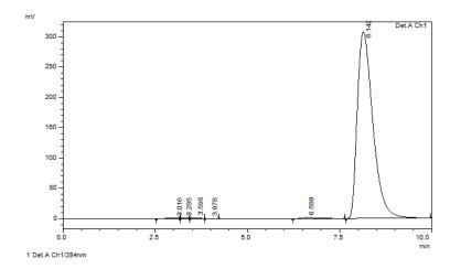
Fig 3 chromatogram showing the retention time for Aceclofenac standard
