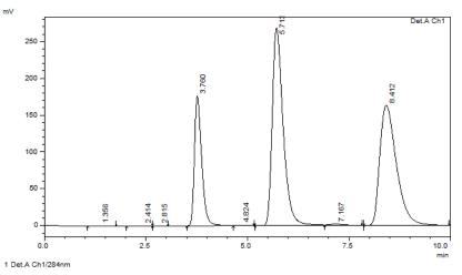
Fig 5 chromatogram showing the combined formulations of Paracetamol, Pantoprazole and Aceclofenac
