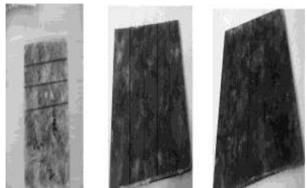
Fig 6: Prepared jute epoxy composite for 85%-15%,80%-20% and70%-30%
