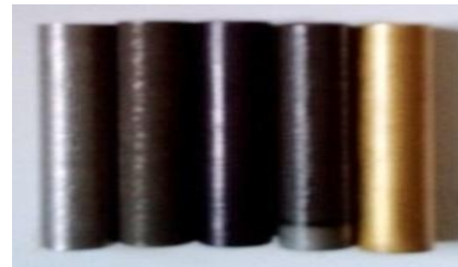
Fig. 4 (a) Wear and COF Test specimen of AISI 4140, (b) Nitrided AISI 4140, (c) Nitrided and TiAlN Coated AISI 4140, (d) Nitrided and WCC Coated AISI 4140, (e) Nitrided and TiN Coated AISI 4140
