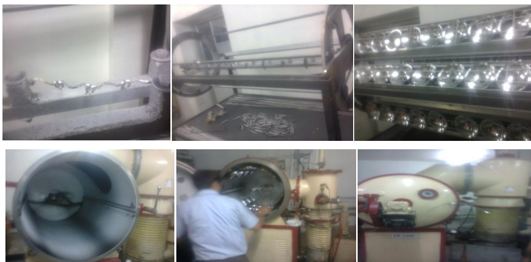
Figure 1 Shows metalizing process
