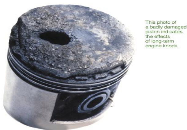
Fig.5. Effect of knocking in piston
