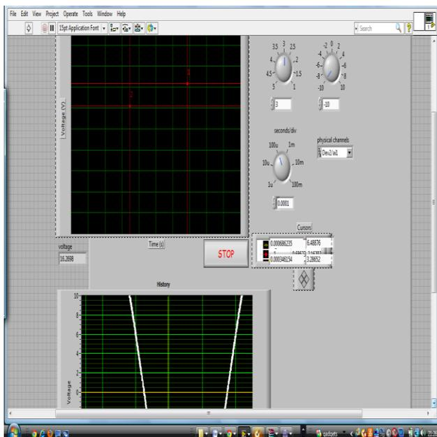
**Figure 2:** front panel diagram of oscilloscope
