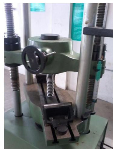
Fig 2: compression test of spring
