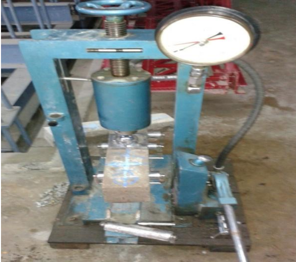
Figure 5: Actual Flexural Loading
