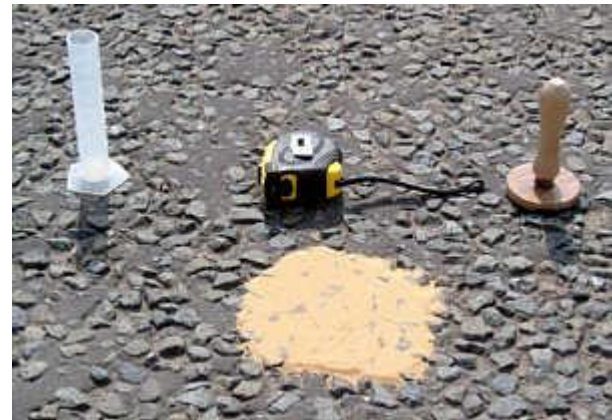
Fig.7 Sand-patch method of measuring texture depth Texture depth = (Volume of sand / Area of sand)
