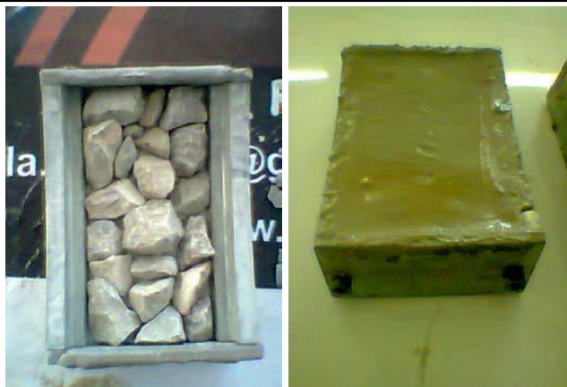
Fig.9 Aggregates placement and preparation in Mould
